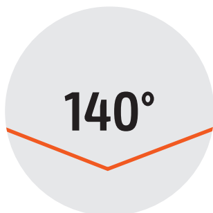
Affilatura frontale a 140°. 140° front sharpening.
